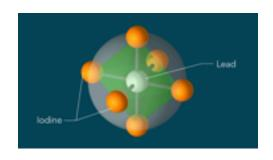
**This** architecture is common to many of the perovskites investigated for solar cell applications. "Previous studies have mostly explored the role of the methylammonium ions and their motions in transporting electric charge through the material," Wu said. "However, we've discovered that light causes large deformations in the network of lead and iodine atoms that could be crucial for the efficiency of perovskites."
